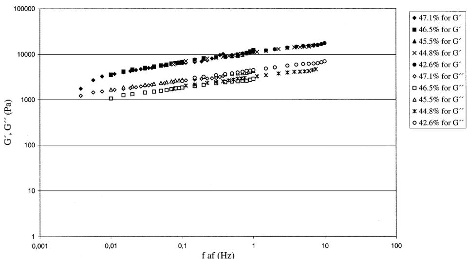
Fig. 5. Master curves of storage modulus ( $G'$ ) and loss modulus ( $G''$ ) for doughs with different water content (42.6–47.1%). The dough with 42.6% is the reference dough.
