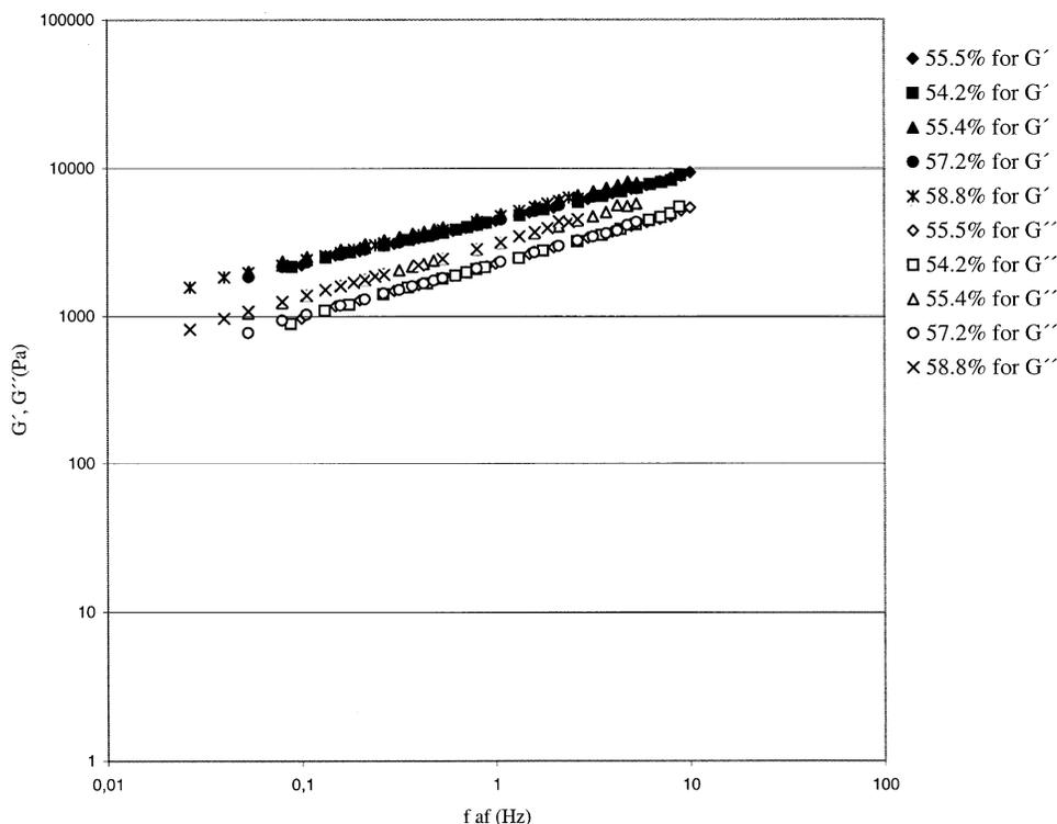
Fig. 4. Master curves of storage modulus ( $G'$ ) and loss modulus ( $G''$ ) for gluten with different water content (55.5–58.8%). The gluten with 55.5% is the reference gluten.
