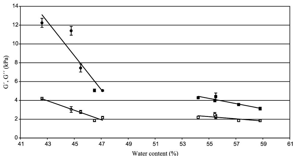
Fig. 2. Storage modulus ( $G'$ ) and loss modulus ( $G''$ ) for dough and gluten, respectively, at different water contents. Data were obtained at a frequency of 1 Hz.  $G'$  for gluten (■),  $G''$  for gluten (□),  $G'$  for dough (●),  $G''$  for dough (○).
